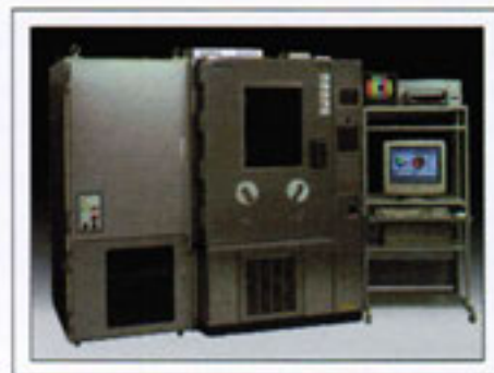
Fig. 6: Otsuka Electronics' LCD-7000 LCD characterization system can accommodate a display of 410 × 256 × 60 mm, and can measure voltage threshold, contrast ratio, response time, spectra, and chromaticity/luminance/color difference.
