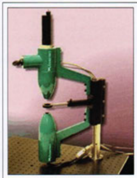
Fig. 5: Axometrics's polarization-measurement system allows the Mueller Matrix Polarimeter instrument to obtain a complete Mueller Matrix of any sample, which completely describes its polarization properties.
