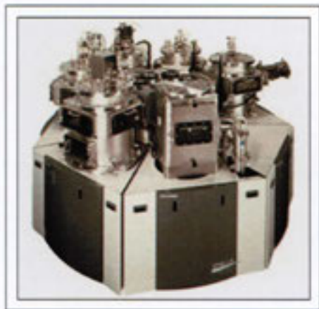
Fig. 3: Ulvac Technologies' Satella OLED cluster tool performs all production steps including OLED evaporation and encapsulation.
